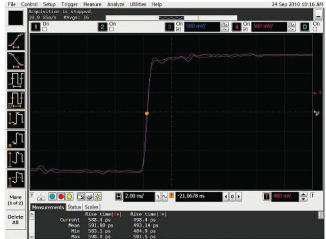
Time domain step response of N2796A (with Keysight MS09404A)
